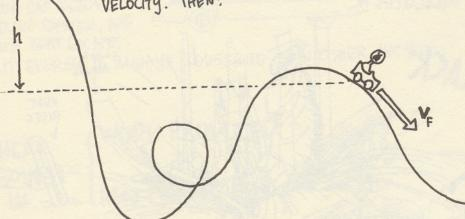
INITIAL ENERGY = ½ mv2 + mgh FINAL ENERGY = ½ mv<sub>F</sub><sup>2</sup> THESE ARE EQUAL, BY CONSERVATION OF ENERGY.  $\frac{1}{2}mV_F = \frac{1}{2}mV_0^2 + mgh$ , 50  $V_F = \sqrt{V_0^2 + 2gh}$  CONSERVATION OF ENERGY TELLS US THAT THE TOTAL ENERGY OF THE SYSTEM DOES NOT CHANGE — BUT THE ENERGY MAY
