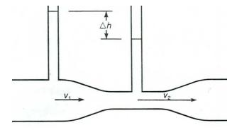
The tube is inserted into a pipe and the difference in pressure between the thick and thin sections of the pipe can be used to determine flow rates. If a venturi tube of  $A_1 = 1.0 \text{ cm}^2$  and  $A_2 = 3.0 \text{ cm}^2$  measures a difference in height of 5 cm (the liquid is water),
