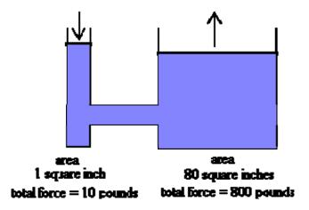
Hydraulic devices make use of Pascal's principle by using small forces to generate much larger ones. A piston of small area is pressed into a fluid at a point of narrow area within a container, which increases the pressure within the fluid by an amount equal to  $F_{in}/A_{iin}$ . The pressure within the entire fluid is increased by this same amount. The force applied to the large piston is then equal to the increase in Pressure multiplied by the larger area  $\rightarrow$
