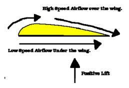
Surfaces that are built in such a way as to cause air to flow faster over one surface than another are called "airfoils". Such surfaces include airplane wings, bird wings, Frisbees, sails, and more. Note that airfoils can also be thought of simply as objects which direct air upward. In pushing air upward, the airfoil itself is pushed downward by the air, in accordance with Newton's 3<sup>rd</sup> law. All examples of Bernoulli's principle can alternatively be understood in this way.
