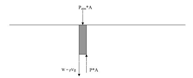
The forces on the column of liquid are the air pushing down from above, the liquid beneath the column pushing up from underneath, and the weight of the column of liquid. Since the forces are balanced,
