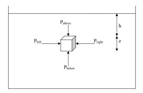
The object has a height of "z", cross-sectional area A, and is "h" meters below the surface of the liquid, which has density  $\rho_{fluid}$ .
