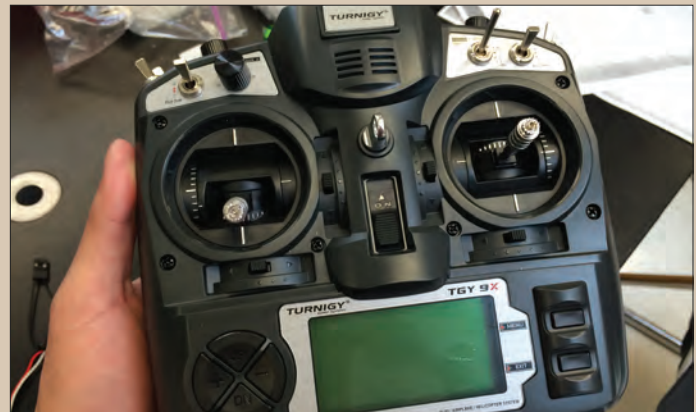
The Turnigy TGY 9X transmitter used to control the quadcopter as a whole.
