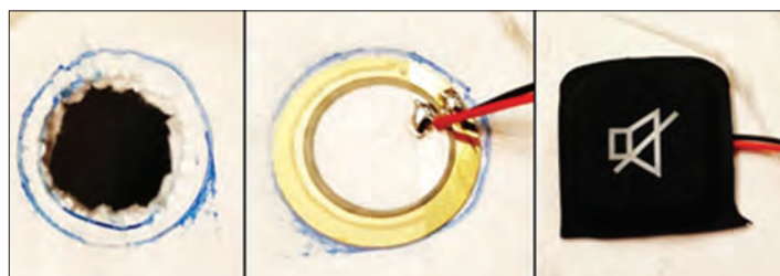
Fig. 4: A foam board with a hole through it, left, a small installed disk and an installed rubber button make up the components of the PZT device.
