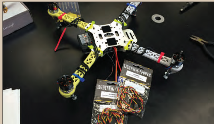
STEP 3: Wires used to connect the motors to the circuit board.
